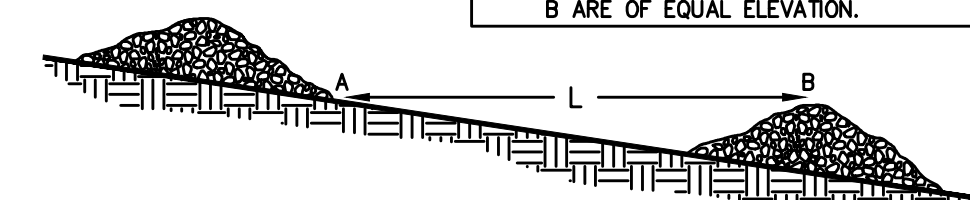
SPACING BETWEEN CHECK DAMS
